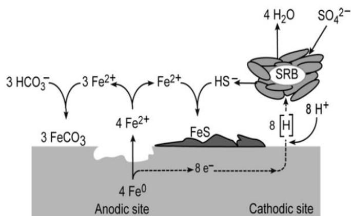
**Figure 1.** Schematic representation of the classical theory of cathodic depolarization by SRB activity (Hang, 2003).
